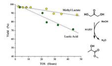
Conversion of dihydroxyacetone and glyceraldehyde to methyl lactate can be achieved in close to quantitative yields using commercially available acidic zeolites. The stability and rate of reaction was found to increase significantly by the use of methanol as solvent when compared to water.
