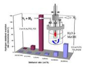
Solar light photocatalytic hydrogen production was obtained from water using low amounts of methanol co-reactant over Pt and  $Au/TiO_2$  (anatase/rutile) photocatalysts, showing the influence of noble metal and porogen promotion.
